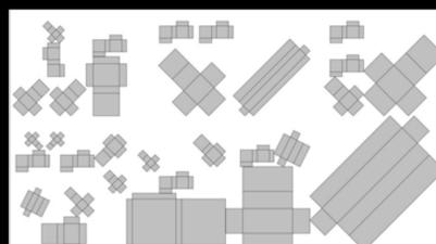
A flattened version of the simplified model, structured for compatibility with vector-based fabrication tools such as laser cutters.
