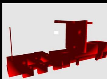
The model is reduced to basic shapes and components. This step enables cleaner unfolding and prepares the layout for 2D transformation.
